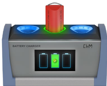
Fig.4. Information about correct, full charge of the battery and completion of charging process
