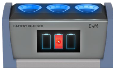
Fig.5. Charging error message or removing the battery before the charging process has finished
