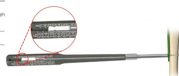
OPTION II: or having removed the threaded guide M3.5/1.8-4.0 [40.4896.018], use depth measure [40.4640.000] to determine the length of the screw.
