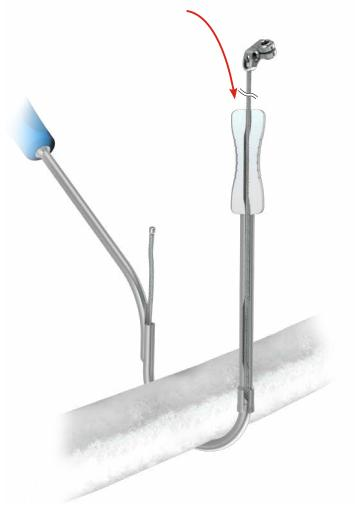
Remove the auxiliary tool - slide the cable through the side channel.
