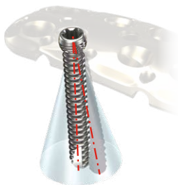
1st screw direction change -INCORRECT
